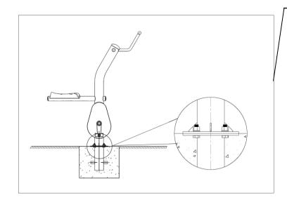
Please be attention: the top of flange must be at the same level or above of ground during process of pouring concrete.
