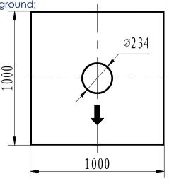
II. Please make sure the centre point of circular, square must comply with the centre point of installation position of each machine in the project diagram.
