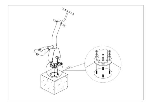
VII. During solidifying of concrete, please be sure the anchor must be vertical to the ground and surface of anchor flange is clear, without weed, soil, detritus cements or even cement mortar.
