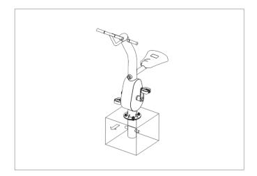
V. Make sure the machine is vertical to the ground and fix well, pour the concrete, and block the space.
