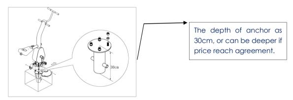
Based on the project diagram, make a circular mark at the center of installation site for each machine, and draw an installation direction by making square mark with sides of 1000mm outside the circular. And dig an embedded hole (with size of Ø234\*300mm) at each marked position of ground;
