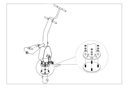
IV. Place the total unit machine onto the installation area & anchor in circular hole, turn the machine around to the installation direction along with the square mark;
