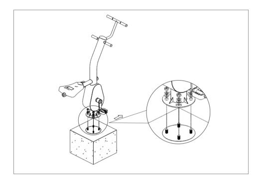
IX. Wingroc will provide one unit plastic case for each 114mm or 89mm upright post fitness equipment. Take apart the case then cover the installation flanges by assembly and fix by tightening bolts and screws.
