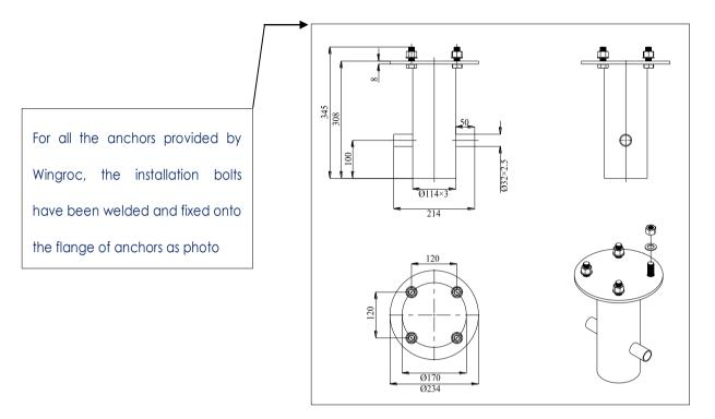
III. Open the package and place the outdoor fitness equipment onto the installation anchors, turn the anchor upon proper alignment of mounting bolts to the mounting holes of machine; each bolt a gasket, spring washer, and lock nut, in turn and then tighten the screws
